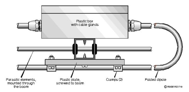
Do **not** attempt to "ground" the middle of a folded dipole to the boom, because that will almost inevitably result in unwanted RF currents running along the boom. The only connection to the boom should be through the balun, allowing the opposite side of the folded dipole find its own electrical centre.
