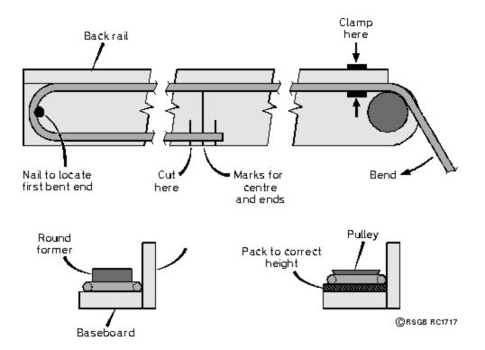
A good way to make the round former would be to use a metal pulley (or a wheel with the rubber tyre removed) because the groove will help to locate the tubing as you bend it. However, the former could be nothing more elaborate than a short sawn-off length of antenna mast, secured to the wooden base of the jig by a few strong nails down the inside.
